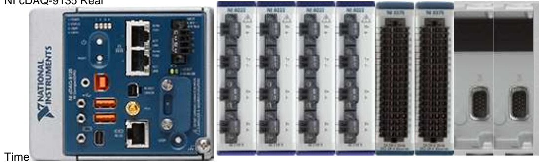
Fig. 5. The front view of the ARS controller [17].
